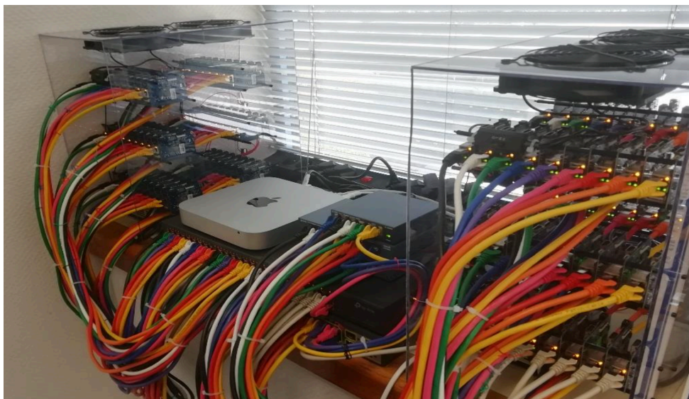
Figure 1. The cluster. Two stacks of Pis on the sides, network switches in the center, and a MacMini as the backend in the centre.
